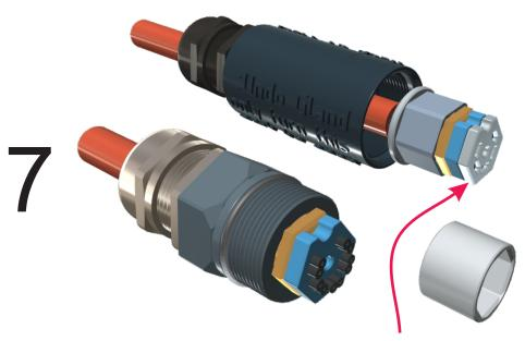
Affix aluminium centre guide to (lower) coupling half shown using the small screw provided. The coupling is ready for joining.
