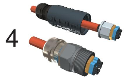
Keep turning the nuts until the face of the brass insert is flush against the back of the threaded insert and the hex flats are aligned
